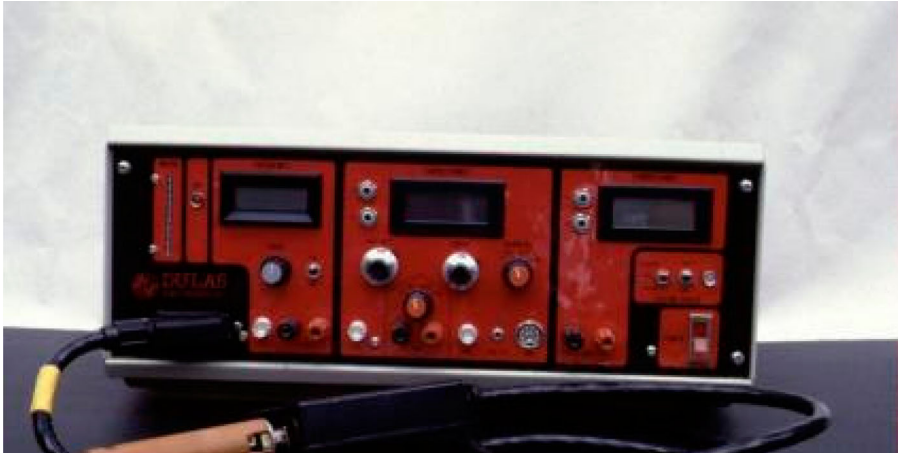
Figure 4. The Biomass Monitor, affectionately known as ‘the Bug Meter’, invented at CAT. Used to electrically measure the volume of respiring biomass in a solution. Undisputably high-tech, and principally used in the brewing industry. Is this AT? Credit: Centre for Alternative Technology.
